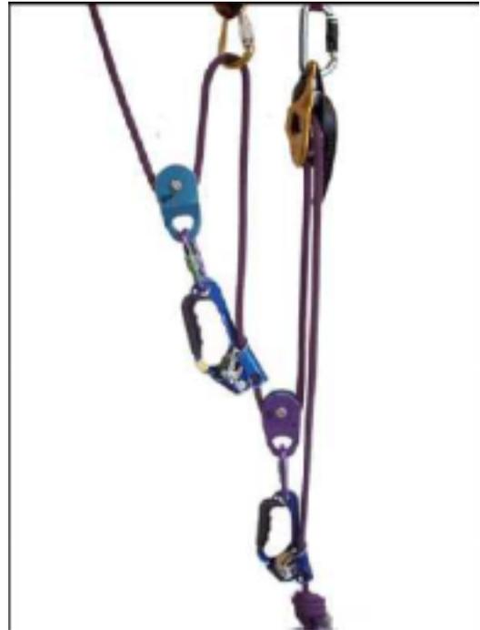
If necessary let several people haul attention that the load does not exceeds 4 kN (coat damage)
