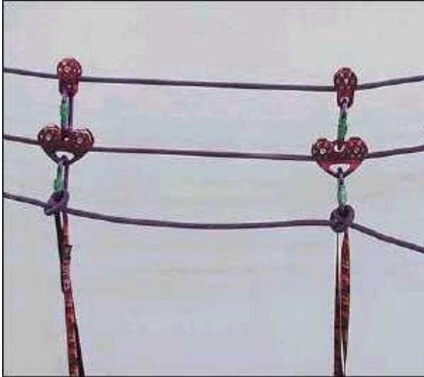
**If possible position the work rope above the safety rope**
