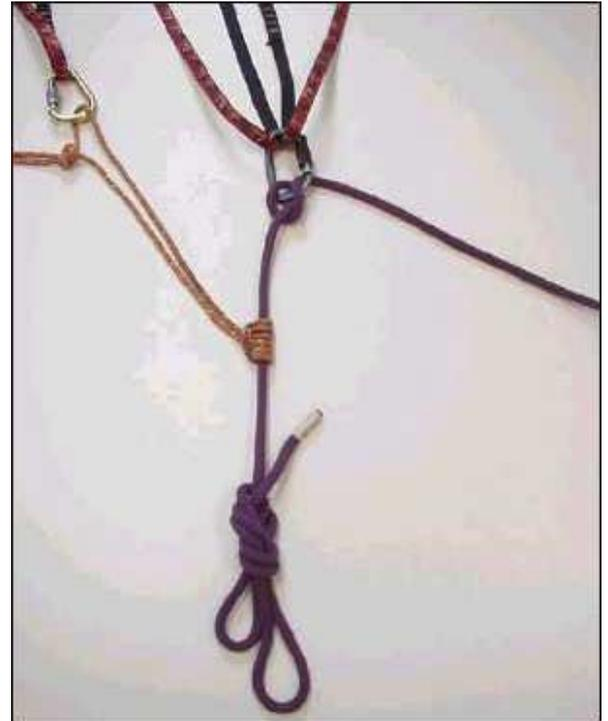
**Position the block knot Machard or prussic at the safety rope on the brake side**
