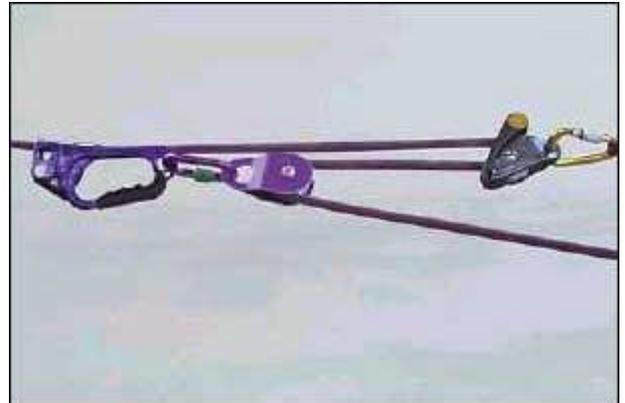
**The Gri-Gri or the HMS-knot need to be backed up via a slip knot**
