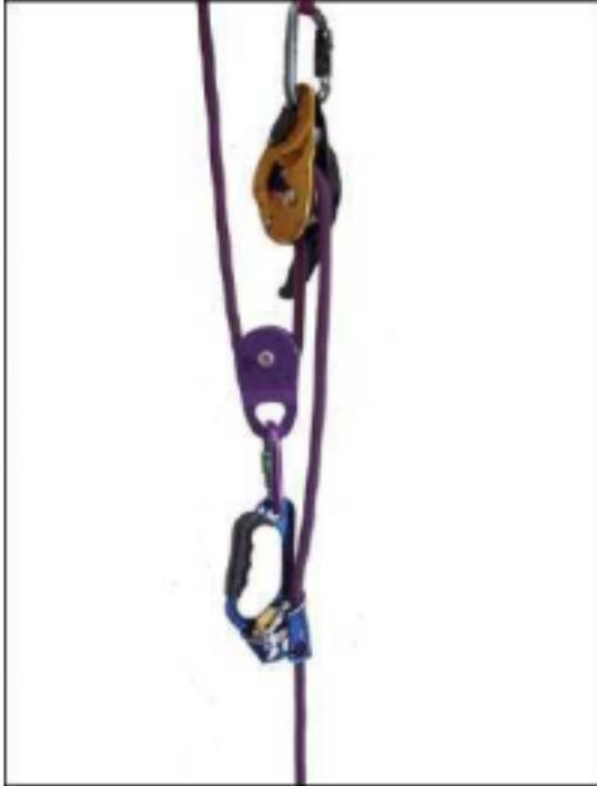
Guide exit rope at the back slip device through pulley
