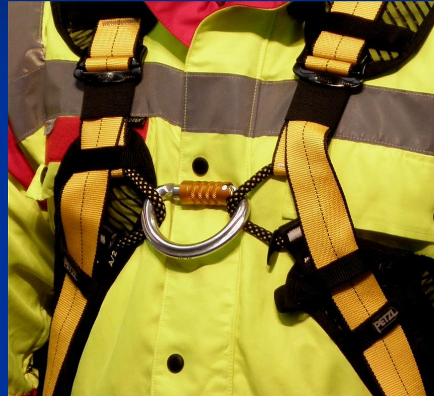
**The connector is put into both attachment loops.**
