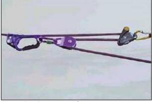
The Gri-Gri or the HMS-knot need to be backed up via a slip knot
