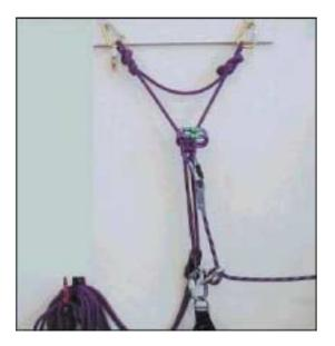
Check that both ropes are independent attached! Is the figure of eight knot made correctly and are all carabiners locked?
