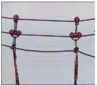
If possible position the work rope above the safety rope
