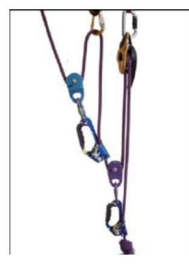
If necessary let several people haul attention that the load does not exceeds 4 kN (coat damage)
