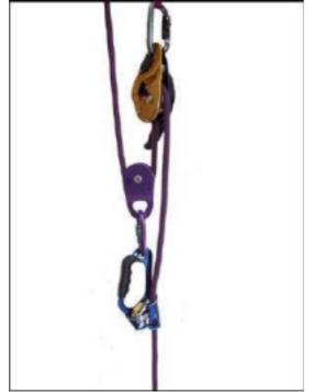
Guide exit rope at the back slip device through pulley
