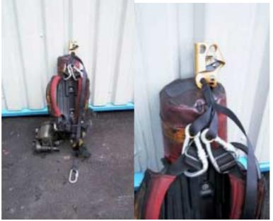
Packaging and supporting the Breathing Apparatus Set in the manner shown, will ensure that the Distress Signal Unit, Contents Gauge and Cylinder Valve are all within the operators reach.
