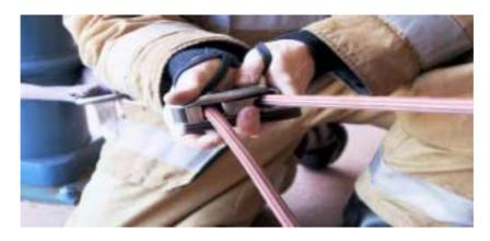
9.2 Once a continuous load has been applied to the Gri-gri, the cam will remain in the locked position.
