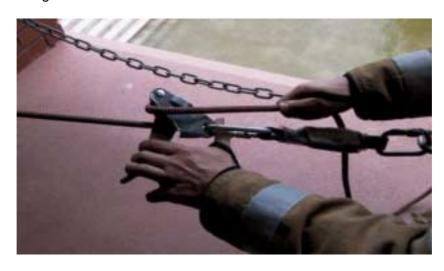
Should the rope pass through the Gri-Gri too quickly, two actions are available to the operator.
